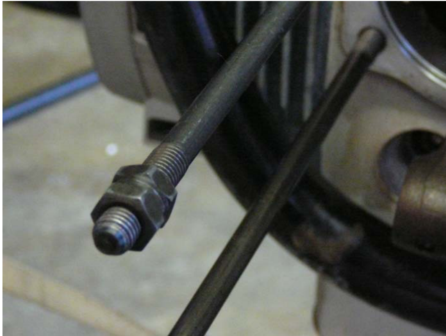
Figure 1: Removal of stripped stud.
