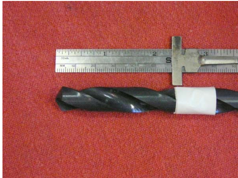
Figure 3: Place a tape marker on drill bit 58mm from tip.
