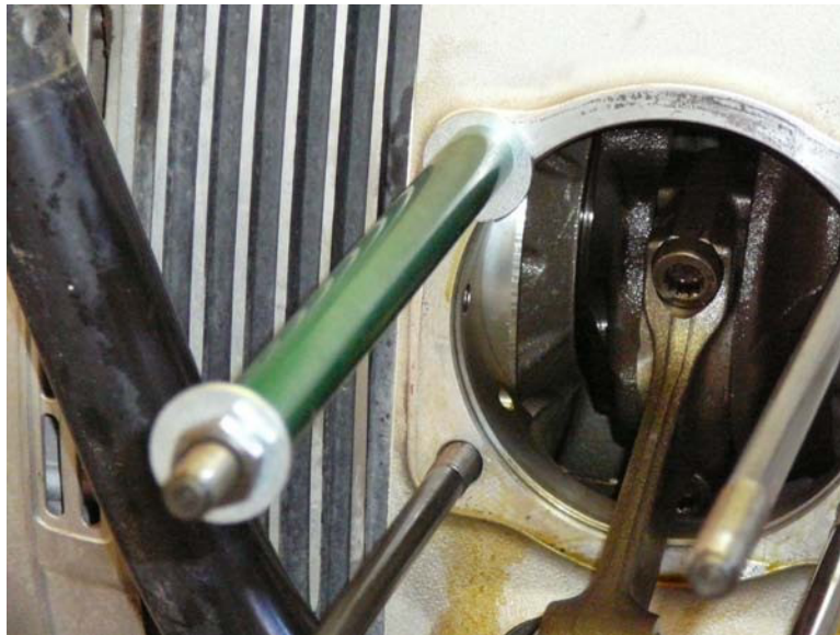
Figure 10: Installation of head stud.
