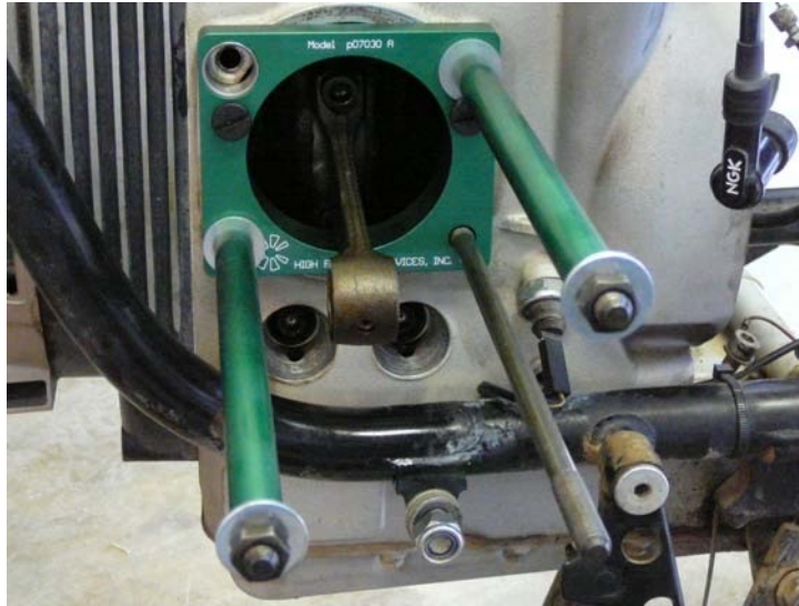
Figure 2: Proper WILLCRAFT Stud Tool installation.
