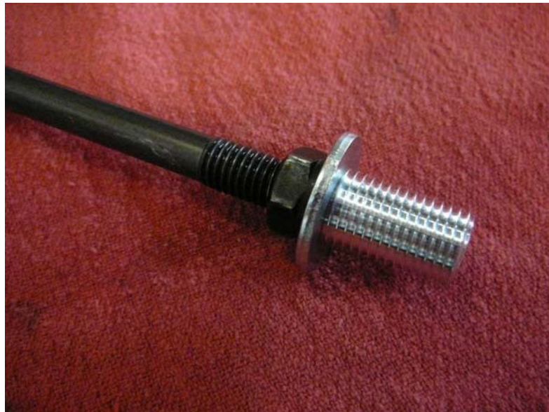
Figure 6: Installation setup for threaded insert.
